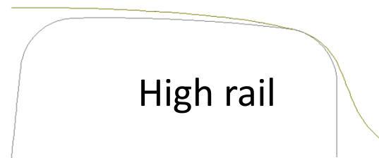
Severe gauge-corner contact
